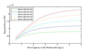
Fig. 11 Thermal power of a single SCA respect to the flow capacity of the molten salts
