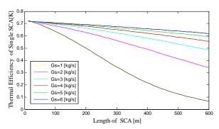
Fig. 10 Thermal efficiency of a single SCA respect to the length of the SCA.
