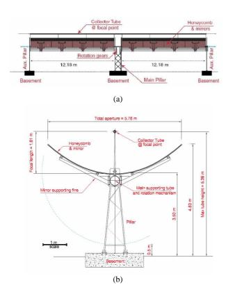
Fig. 1. Reflectors with receiver pipe
