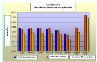
Fig. 5. Comparison between GHI and DNI
