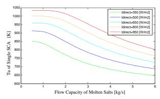
Fig. 8 Thermal performance of a single SCA respect to the flow capacity
