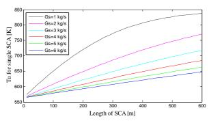
Fig. 9 Thermal performance of a single SCA respect to the length of the receiver
