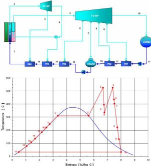
Fig. 3. Thermal cycle (a) and T-E diagram (b).
